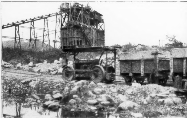
Locomotive Hauling Dump Cars Equipped with Automatic Release Swinging End Doors
